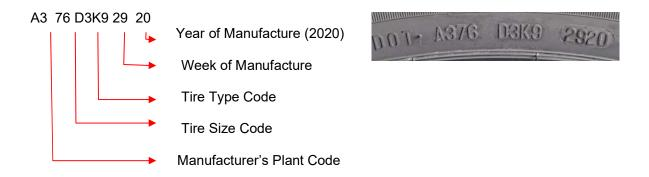
Tires made for use in the United States have a unique mold number located on both sidewalls of the tire.
